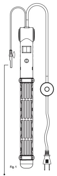
Clean and confirm the out-of-water sensor is functioning properly every 30 days. DO NOT USE heater if out-of-water sensor is inoperative.
