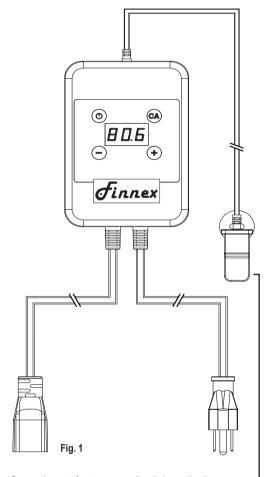
Secure the out-of-water sensor directly beneathe the senor cord clip, without any slack, and above the heating element at all times. Clean and confirm out-of-water sensor is functioning properly every 30 days. DO NOT USE heater if out-of-water sensor is inoperative.
